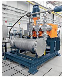
A brand new, state-of-the-art test bench means that ProMinent is able to carry out tests on process metering pumps in accordance with API 675.
