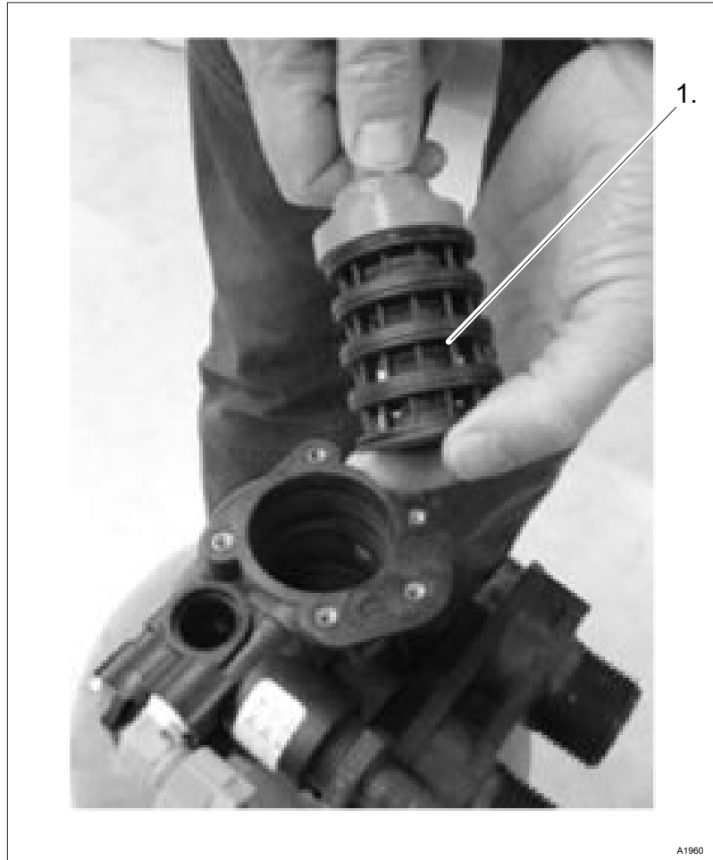
Fig. 21: Greasing and replacing the rubber washers
