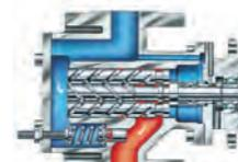
For high or low viscosity fluids with good lubricity.
