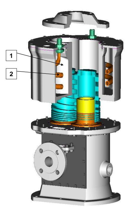
Indirect cooling of the working chamber:
