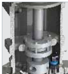
Robust cast-iron bearing housing
