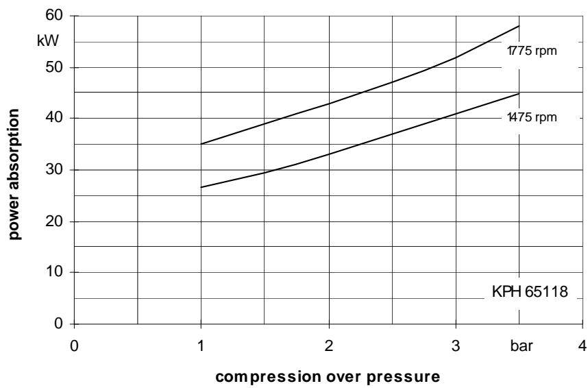
The values indicated for volume and power absorption are valid for compression of dry air at 20°C from atmospheric pressure (1013 mbar) of the respective compression pressure with water at 20°C as service liquid. Tolerance of the curve values is 10%. The compression pressure in bar is indicated as pressure above the atmospheric pressure.
