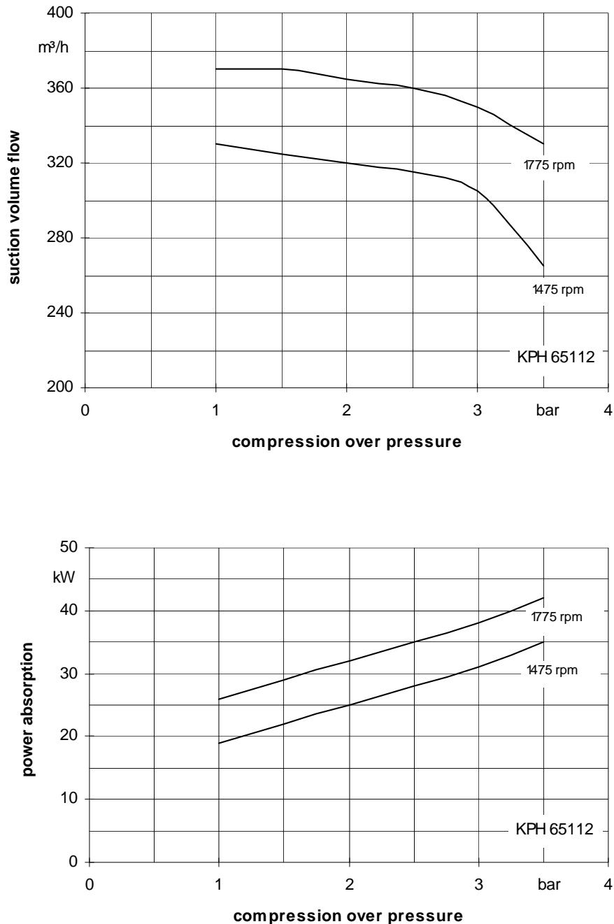
The values indicated for volume and power absorption are valid for compression of dry air at 20°C from atmospheric pressure (1013 mbar) of the respective compression pressure with water at 20°C as service liquid. Tolerance of the curve values is 10%. The compression pressure in bar is indicated as pressure above the atmospheric pressure.
