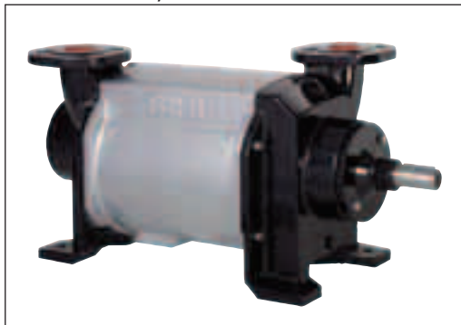
Fig. 1: The Sterling SIHI range of liquid ring vacuum pumps is available in single and two stage designs, with suction capacities up to 12000 m 3 /h and suction pressures in the range 33 to 1013 mbar.
