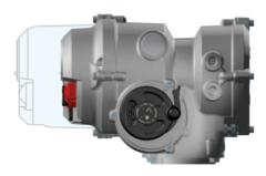
Rotork offer many actuation solutions for specialised apllications. For example, the IQTN (shown above) has been especially developed for use in marine applications where space is at a premium. Rotork have developed this product which now enjoys all the benefits and performance of the standard IQT range whilst reducing the actuators weight and space envelope and increasing its shock resistance.
