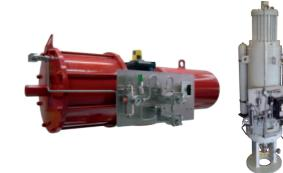
Control component packages are a part of any actuator/valve installation. Rotork has extensive experience in the design and assembly of all types of fluid power control systems to satisfy any customer requirement for on/off, modulating or ESD (emergency shutdown) service. Packages can be mounted on a panel or in a cabinet and mounted either on the actuator or at a remote location.
