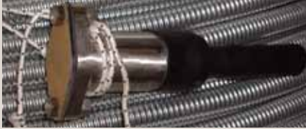
Armored cable with plug motor connection
